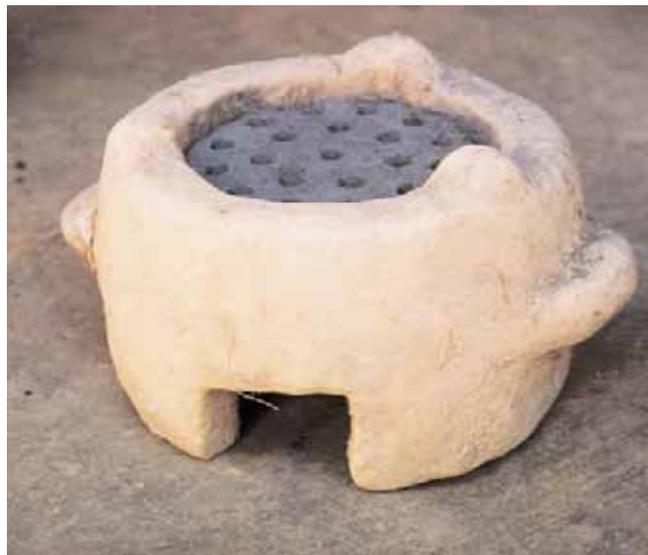
*Honeycomb briquette in specially designed mud stove.*
