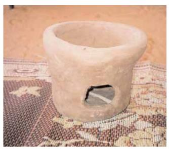
Fuel-efficient stove in Abu Shouk Women's Center, El Fasher, North Darfur. The stoves are made of a clay-sand mixture, animal dung and water, and are built around three horizontal bricks (on which the pot sits). Pots are placed almost fully inside the stove. A single piece of firewood is inserted under the pot through the small "door" at the base of the stove.
