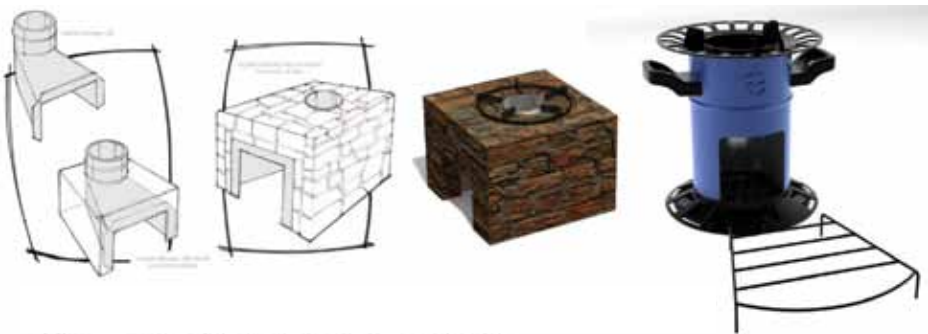
ENVIROFIT INTERNATIONAL - (Left) Schematic and rendering of Envirofit BUILT-IN COOKSTOVE prototype, (Right) Preliminary rendering of Envirofit LOW-COST COOKSTOVE prototype
